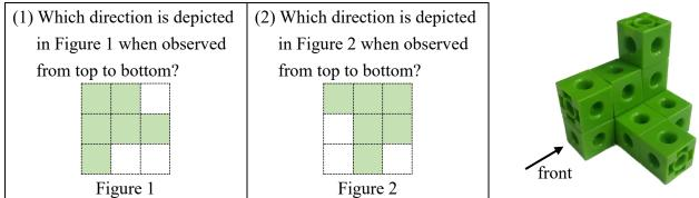
We can find the top view is different if we look from different directions. For the convenience of communication, we define the top view as drawn from the front of the object.
