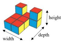
The front view shows the width and height of the object.
